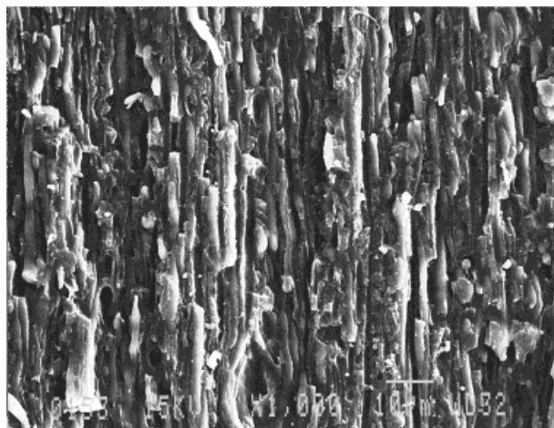
Figure 14 SEM fractographs of injection-molded PBT/PA66/LCP42.5/42.5/15 composite.
